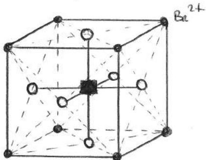
$$\begin{aligned} \text{Ba}^{2+}: & \bullet \rightarrow 8 \times \frac{1}{8} = 1 \text{ Ba}^{2+} \\ \text{O}^{2-}: & \circ \rightarrow 6 \times \frac{1}{2} = 3 \cdot \text{O}^{2-} \\ \text{Ti}^{4+}: & \blacksquare \rightarrow 1 \times 1 = 1 \text{ Ti}^{4+} \end{aligned} \quad \left. \right\} \text{BaTiO}_3$$
